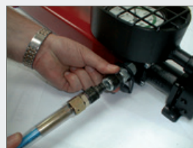
Hand Pump is fitted with an high pressure female coupling
