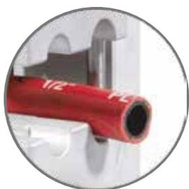
**1** Insert the hose into the suitable groove in the hose housing and rotate the hose handle to clamp the hose down.
